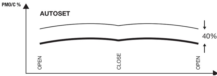
The default value at 40% is normally enough to avoid false interventions. In any case, if PMO and PMC should be modified, the impact tests set out by regulations in force will have to be carried out.
